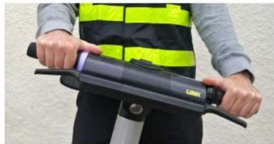
No cables are exposed on the LINK scooter, protecting them from tampering and vandalism.
