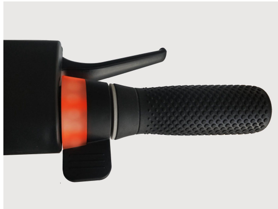
When parking in a No Parking Zone, red LEDs on the handlebar flash, front and tail lights flash, and the speaker plays an alarm tone every 10 seconds
