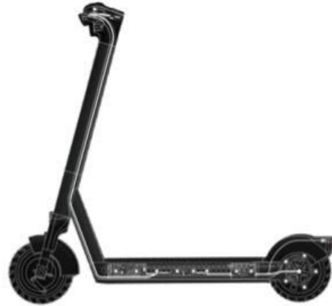
The LINK VIS has 5 microprocessors and nearly 75 sensors throughout the scooter, helping to keep the rider and the public safe.
