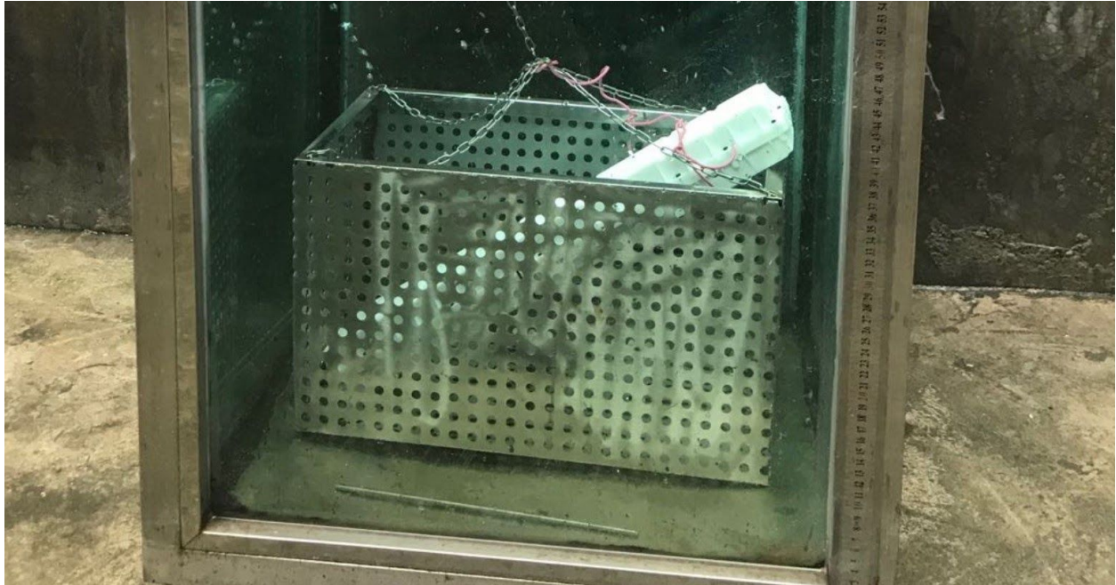
Snapshot from some early LINK scooter immersion testing.
